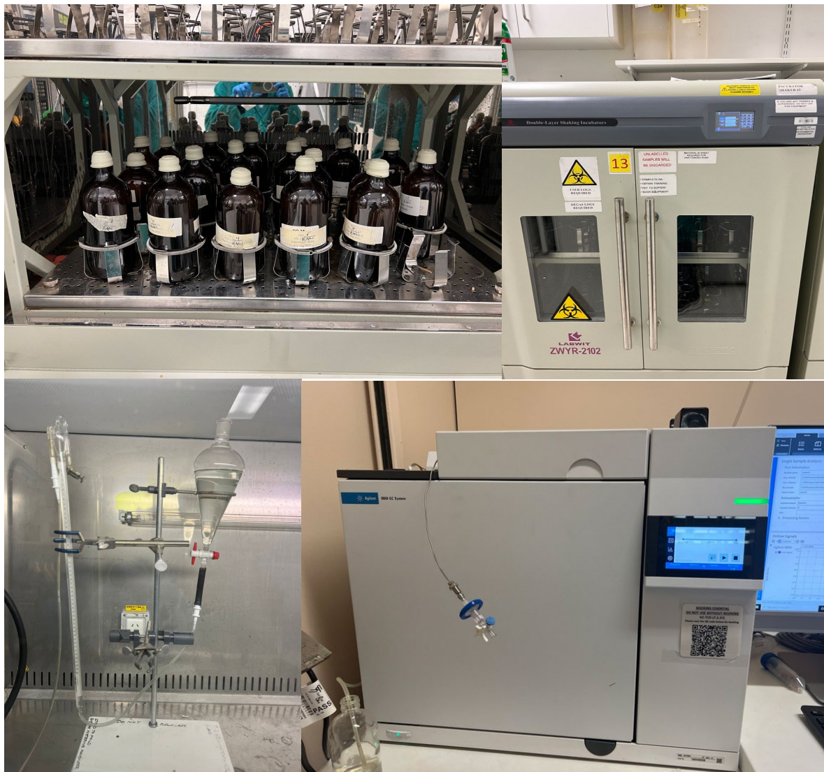
Figure 2: Apparatus of the anaerobic digestion experiments, including (top) the test bottles in the incubator, the closed incubator, and (bottom) the water displacement manometer and GC used to measure biogas volume and composition. Source: Tabatabaei (2025).
